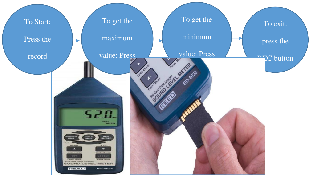
Figure 2: Sound level meter (noise instrument)
