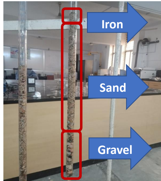
Figure 2: Filtration to separate As and iron from the water.
