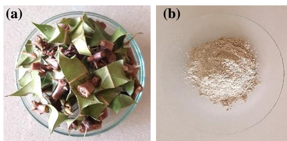
Figure 1 Stem and leaves of A. mexicana (a) and equipped adsorbent of from A. mexicana (b)
