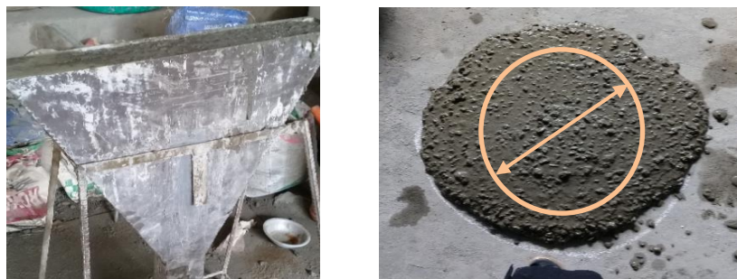
Figure-4: Trial mix SF-7.5 (a) Slump flow test, (b) V-funnel test
