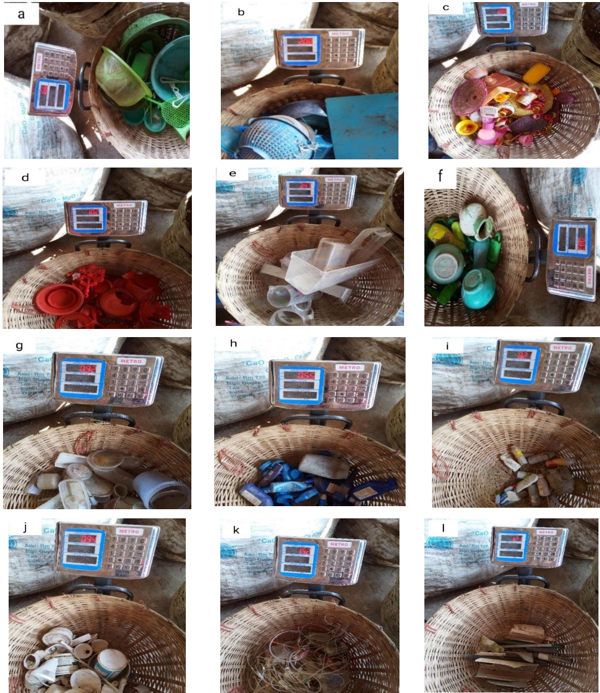
Figure 5: Grades of plastic waste in the recycling shops: (a) Green PP, b) Blue PP, c) 1 No PP, d) Red RFL, e) Hard Pipe, f) Green Hybrudge, g) Water PP, h) Blue Hybrudge, i) Pran Product, j) Milk PP, k) saline Lota, l) Hard Water Pipe (Photographer: Md. Kawsar Ahmed, 2022)
