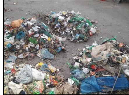
Figure 4: Quarter method for solid waste sample (Tariqul, 2022)
