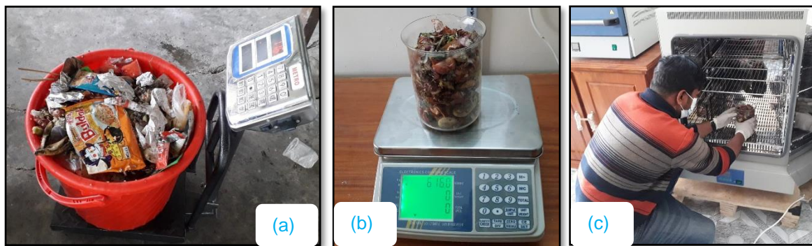
Figure 6: Taking the wet weight of MSW and oven dry at waste laboratory KUET (Noman, 2022)
