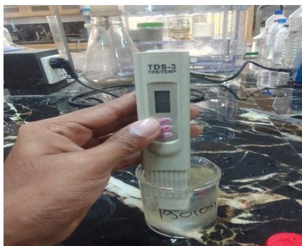
Figure 5 Total Dissolved Solids Test.
