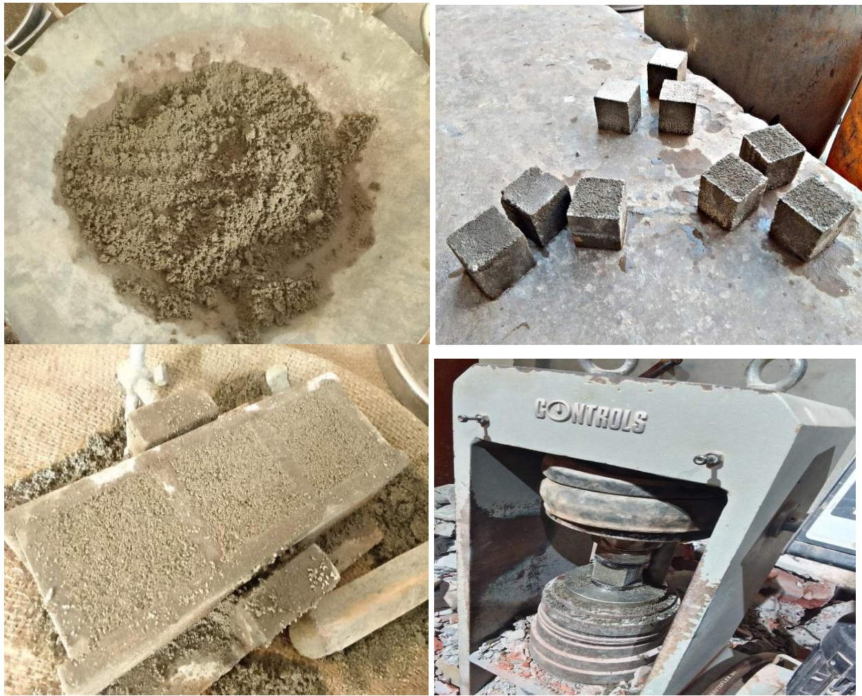
Figure 9 Casting and compressive strength testing of mortar.
