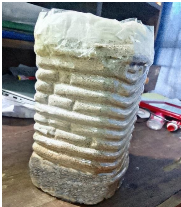
Figure 2 The slow sand filter
