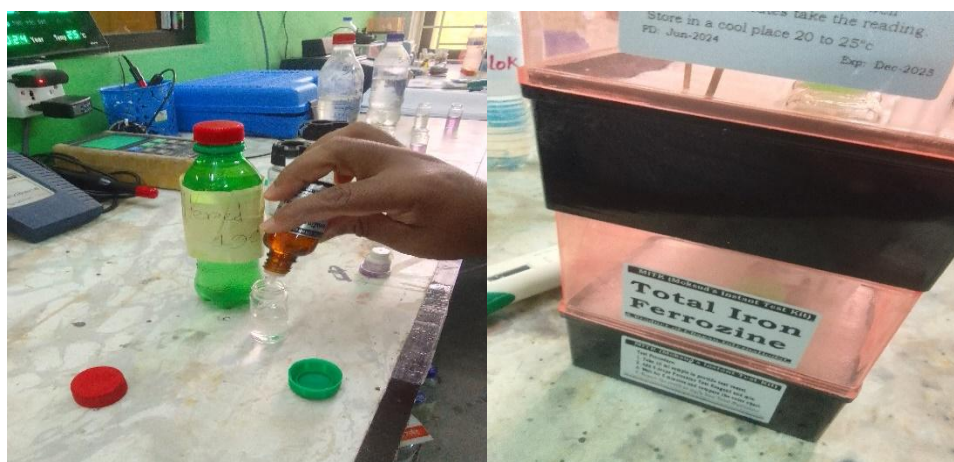
Figure 4 Iron and Manganese conc. Test
