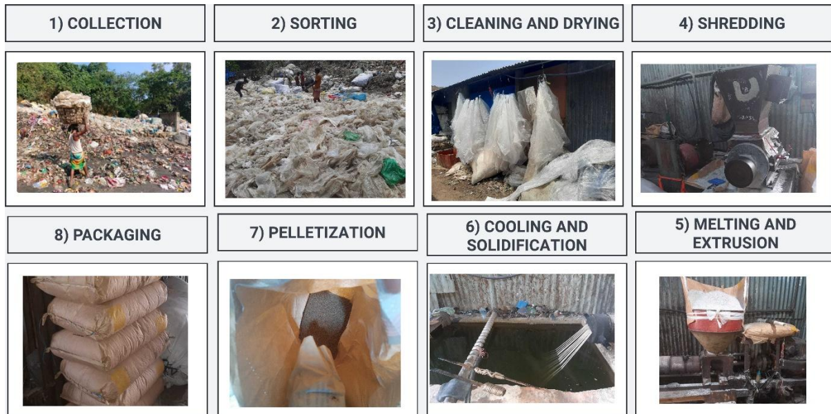
Figure 6 Typical step-by-step process of plastic recycling
