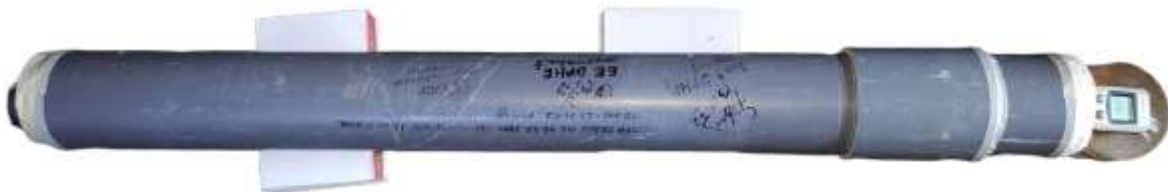
Figure 5. Experimental setup for impedance tube method.
