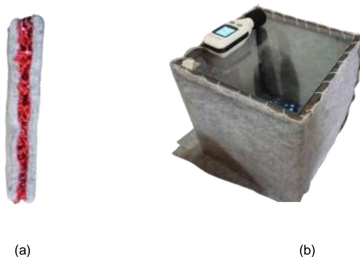
Figure 4 (a) Geotex-Foam-Geotex composite structure. (b) Experimental setup for closed enclosure.
