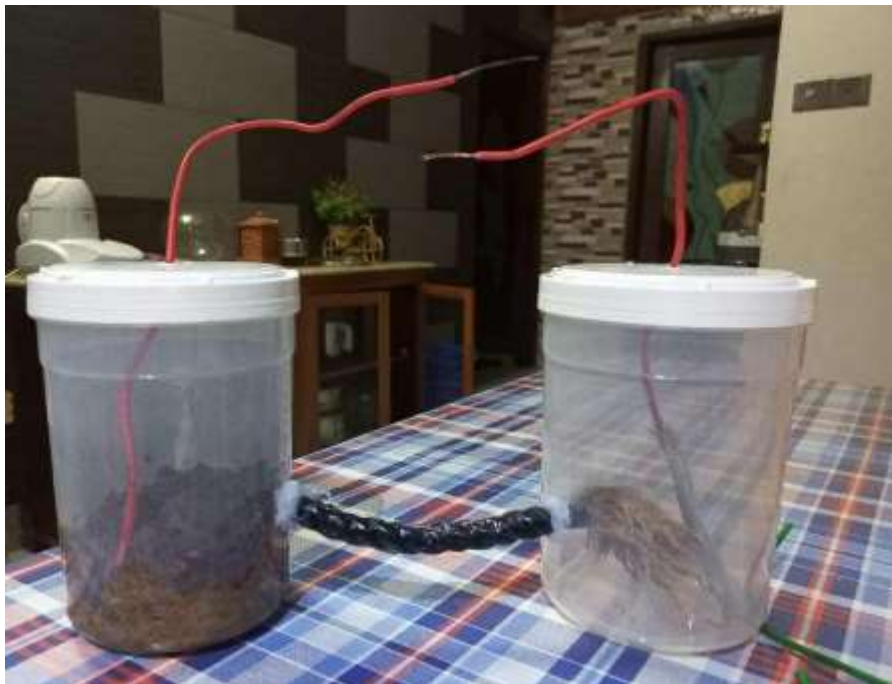
Fig. 5: Electricity Production Experiment by Kitchen Waste using MFC
