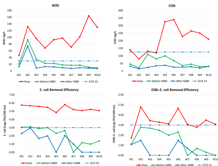
Figure 1 BOD, COD, E. coli and ESBL- E. coli results in treated effluents
