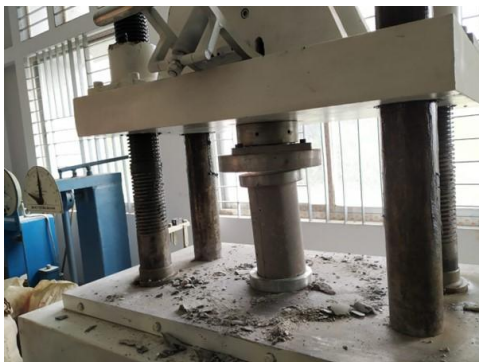
Figure 4 Test setup for compression test of cylinders
