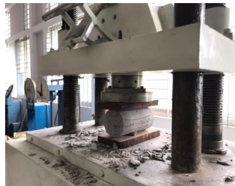
Figure 5 Test setup for splitting tensile strength of cylinders
