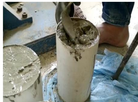
Figure 2 Filling the cylinder sampler with concrete for test
