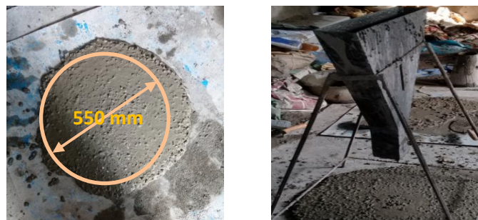
Figure-2 Control mix (a) Slump flow test, (b) V-funnel test
