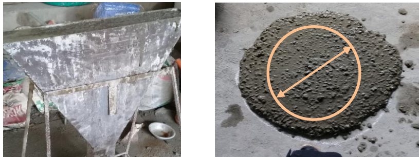
Figure 4 Trial mix SF-7.5 (a) Slump flow test, (b) V-funnel test
