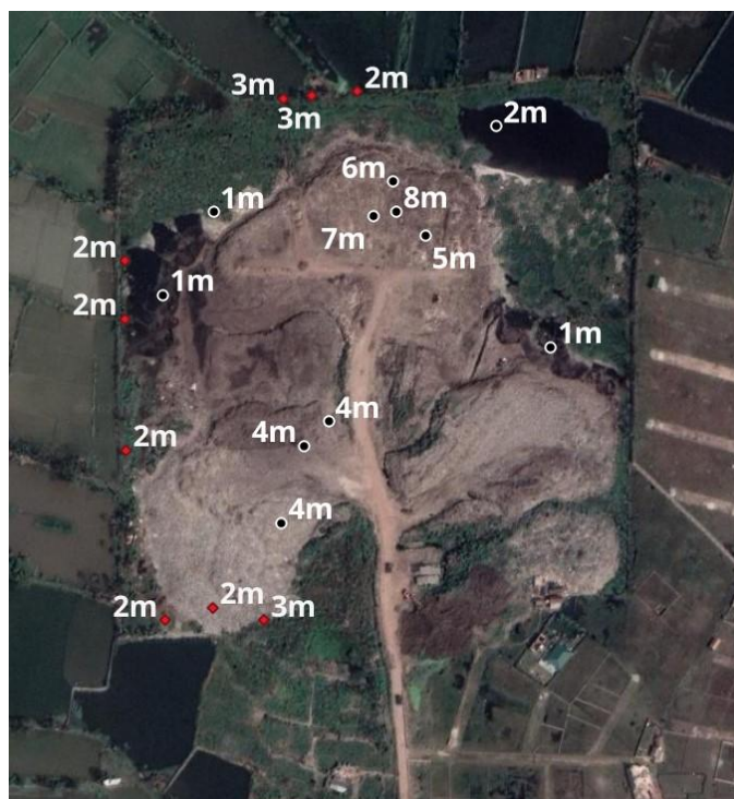
Figure 28 Elevation of different points in the site (QGIS with Google Earth Pro, 2022)
